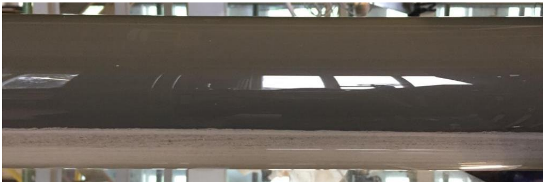
Figure 5. 3 Layering of particles at the bottom of the pipe, clear horizontal section; no flow condition. Overall, the effect of inclination in the particles' distribution in the pipe is significant. The change is considerably higher in negative slopes, where the flow is fully stratified.
