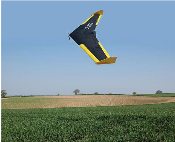
Figure 3. A fixed-wing drone, reprinted from https://www.circuitstoday.com/types-of-drones
