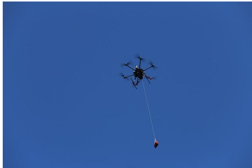
Figure 18. Drone delivering an AED, reprinted from https://uavcoach.com/everdrone-defibrillators/
