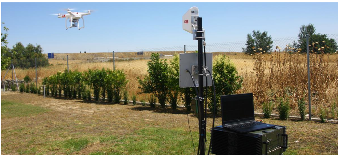
Figure 11. GPS spoofer sending a new signal to the drone, reprinted from https://www.robinradar.com/press/blog/9-counter-drone-technologies-to-detect-and-stop-drones-today
