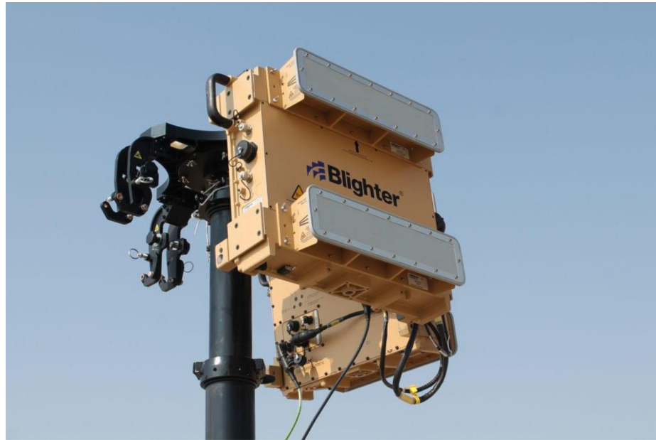
Figure 9. A radar used against low-flying drones, reprinted from https://www.unmannedsystemstechnology.com/2019/09/counter-drone-radar-enhanced-against-low-flying-and-small-uas/
