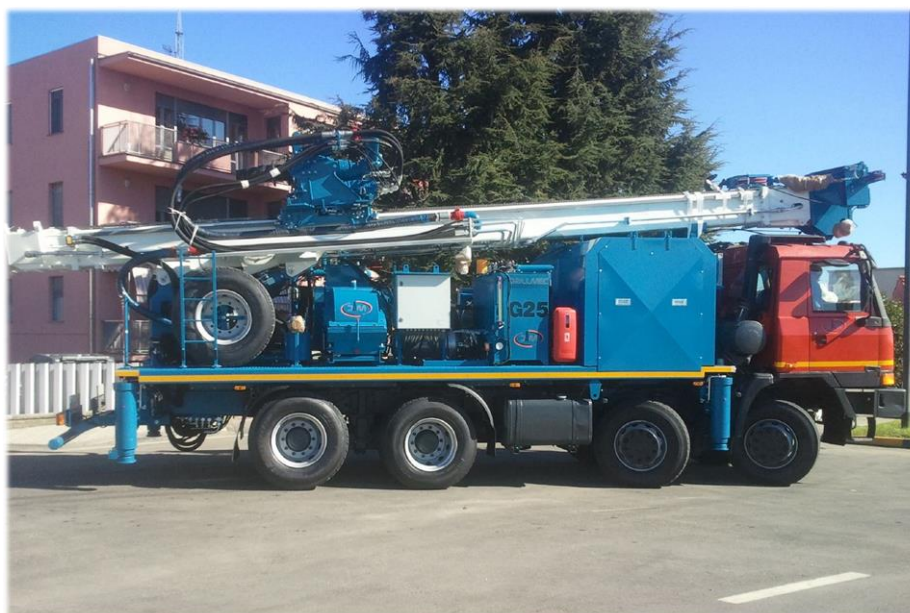
Obr. 6.2 Vrtná souprava DRILLMAC G 25 [16]
