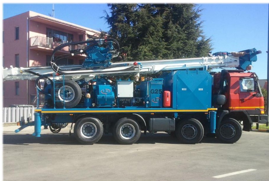
Obr. 6.2 Vrtná souprava DRILLMAC G 25 [16]
