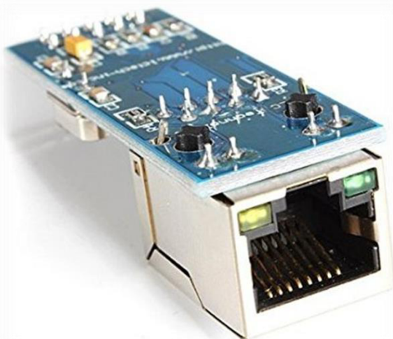
Obr. 31: Modul Ethernet shield ENC28J60
