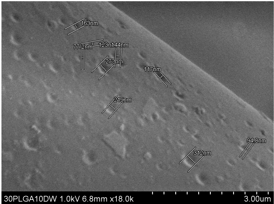
Figure 30. SEM image of 30 % (w/w) PLGA fibres incubated in distilled water for 10 days at the temperature 42 °C.
