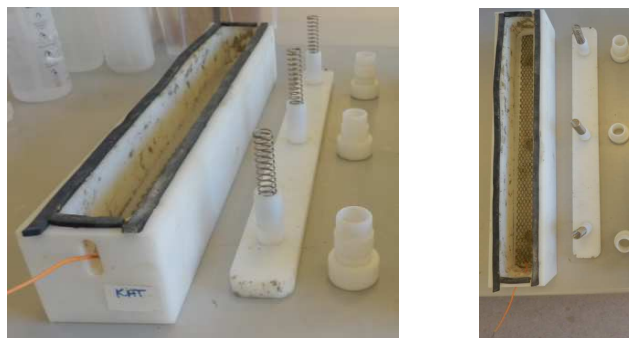
Fig. 61 The electrode unit – the movable bottom, the mesh electrode, the springs, the plastic heads, the rubber tape band.
