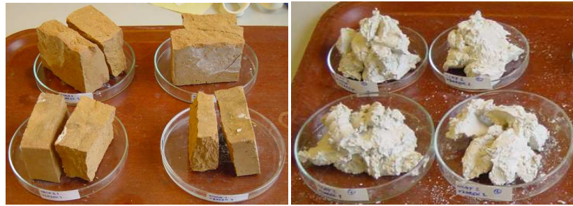
Fig. 16 The segmented parts, where the water contents and pH were measured. L1 – the clay poultice, L2 – half of the brick;
