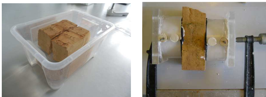
Fig. 54 The used yellow brick contaminated with NaCl solution (left) and the used closed laboratory setup (right). The wrapping is not shown. [39]
