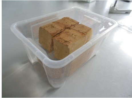
Fig. 17 The halves of the brick submerged in the tap water for two hours.
