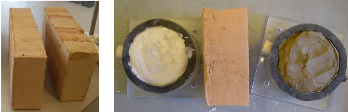
Fig. 14 The used yellow bricks, the clay poultices – the mixture (white), the brick clay (brown); [33]
