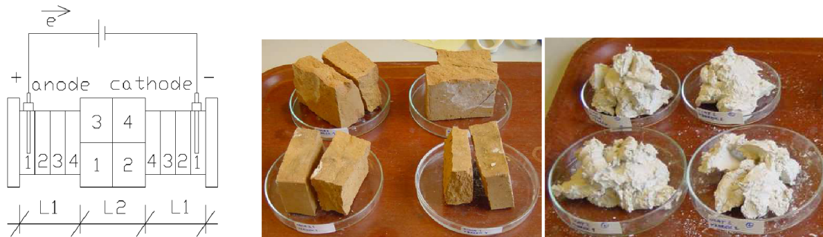
Fig. 16 The segmented parts, where the water contents and pH were measured. L1 – the clay poultice, L2 – half of the brick;
