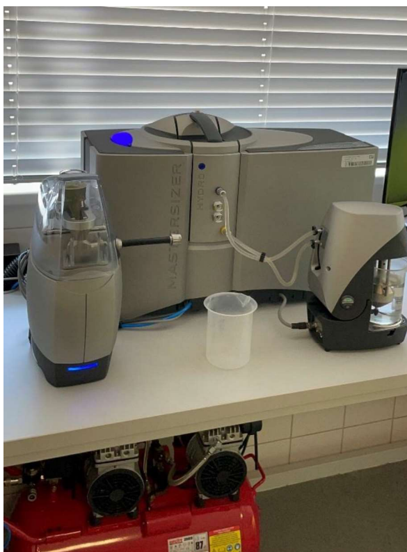
Figure 8: Malvern Mastersizer 3000 equipped with Hydro unit
