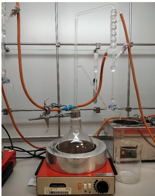
Figure 3. The Clevenger type apparatus (Merci, Prague, Czech Republic) (Gábor 2023)
