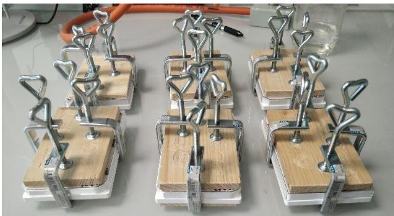
Figure 5. Plates and lids fastened together using clamps and wooden pads (Gábor 2023)
