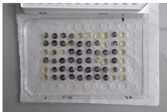
Figure 7. Determination of MIC on the lid of the 96-well microtiter plate (Gábor 2023)
