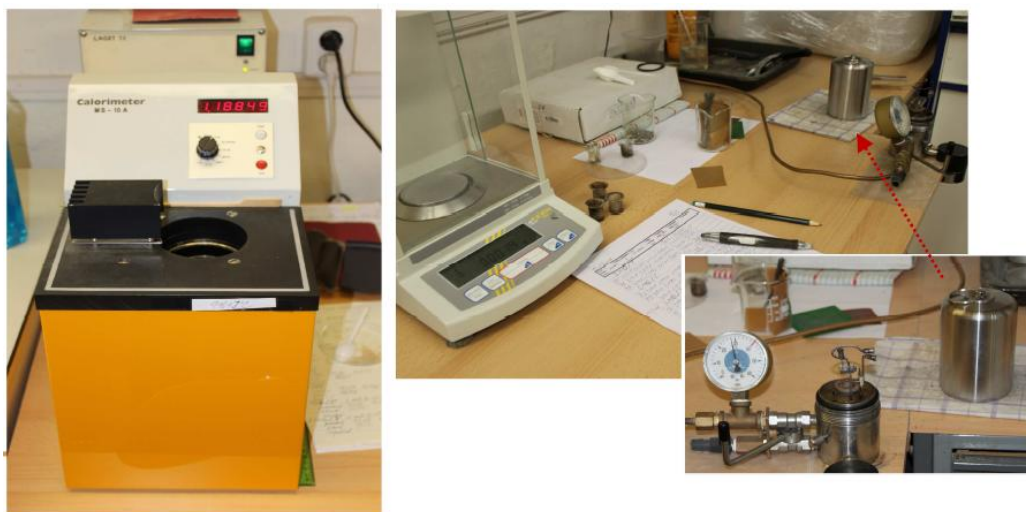
Fig. 13 – The bomb calorimeter MS – 10A (left) and calorimetric bomb, oxygen pressure gauge, slot for the calorimetric bomb placement and laboratory scale KERN ABJ (right) (IVANOVA, 2012)
