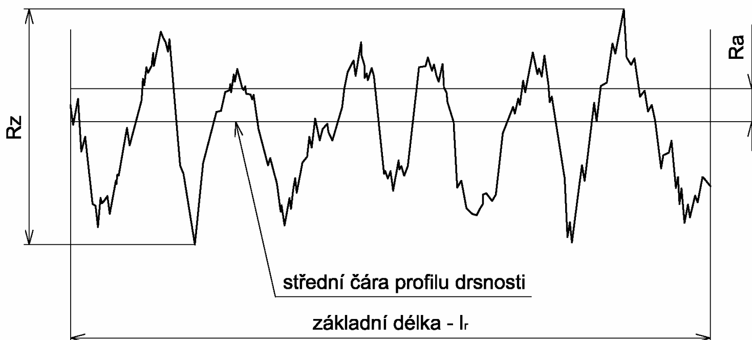
Obr. 4.3 Parametry drsnosti R_a a R_z [66]
