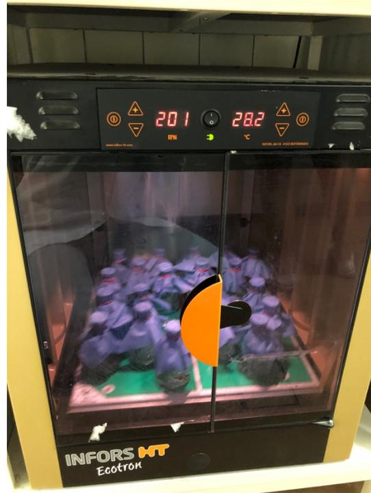
Figure 4a (left): Sterilized 250ml Erlenmeyer flasks filled with liquid medium, ready to be planted with bacterial cultivars grown in agar solid medium. (photo by author, 2020).
