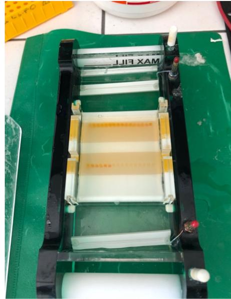
Figure 7 (left): On a photo is an assembled gel stand with rubber sides and combs, already filled with gel solution.
