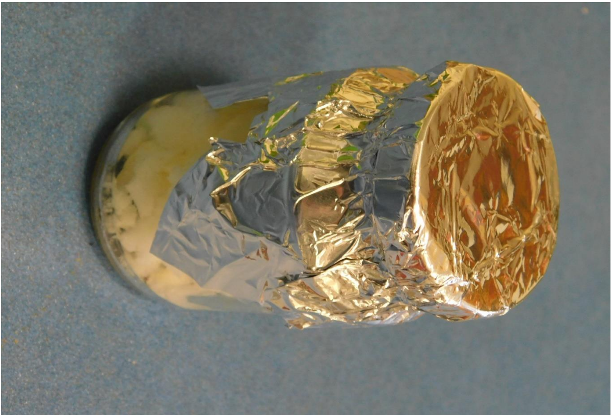
Figure 4 Look of the finished liquid culture flasks with polyurethane foam
