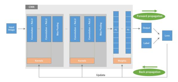
Fig. 1.2: A CNN architecture and its training process. Source: Adapted from [10].
