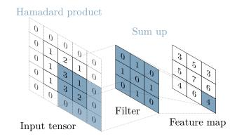
Fig. 1.3: An example of convolution with zero padding. The filter size and the stride are set to  $3 \times 3$  and 1.
