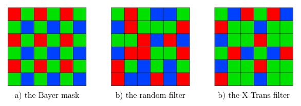
Fig. 4.2: Different color filters used in experiments.
