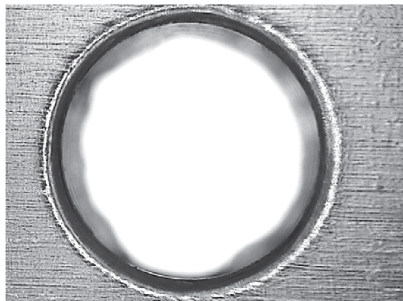
Figure 8.17: Photograph from hole entry side of Figure 8.16. Unfinished full drill diameter at the hole exit.
