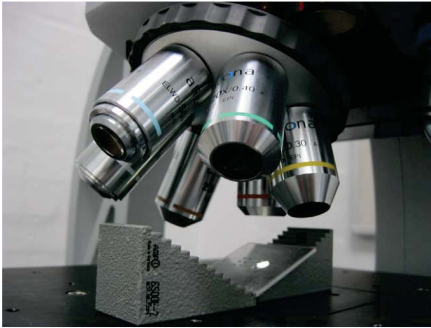
Figure 6.24: Workpiece clamping by means of stair-step fixture on Alicona Infinite-focus working table.
