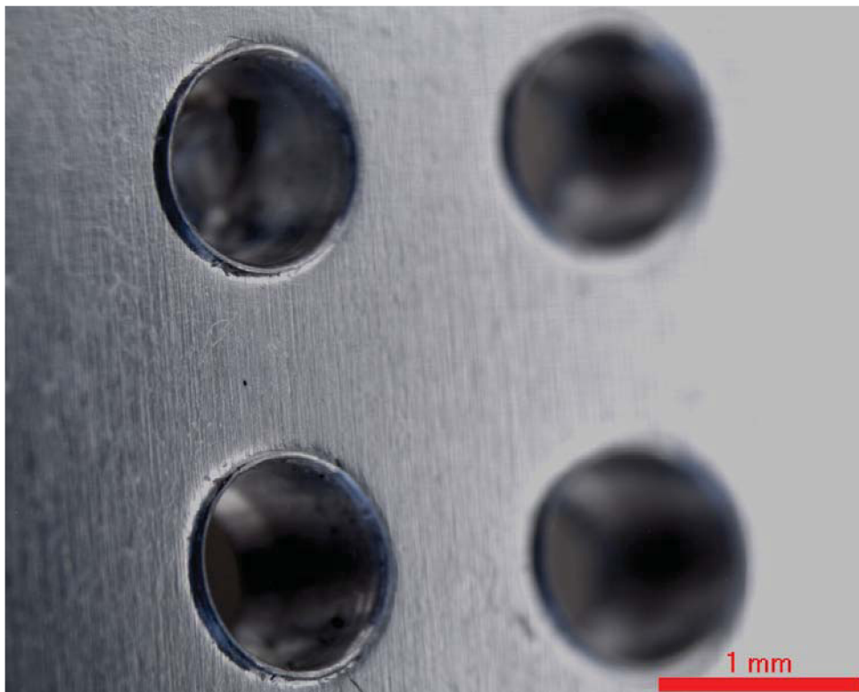
Figure 8.15: Photograph of hole entry burrs, Drill A, 1st setting ( v_c = 226 \text{ m} \cdot \text{min}^{-1} , f = 0.190 \text{ mm} ).
