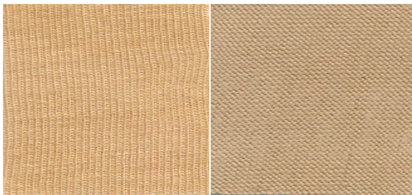
Figure 17: Example of excellent brown color hues of D3 (left) and D9 (right) lignite humic acid direct azo dye on cotton fabric at 80°C by Nasir et al. [184].
