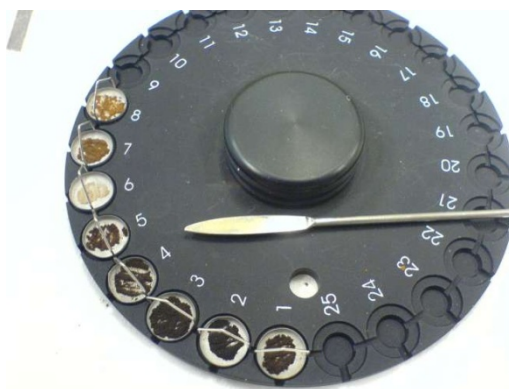
Figure 29: Humic acids (HA)(1–5) and filtrates (RFILT)(6–8) samples on the Q5000 autosampler carousel in Pt pans.
