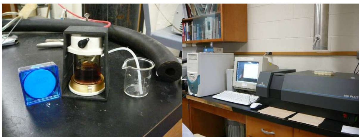
Figure 30: Amicon filtration device with humic sample (left) and the Coulter N4 Plus Submicron Particle Sizer (right).
