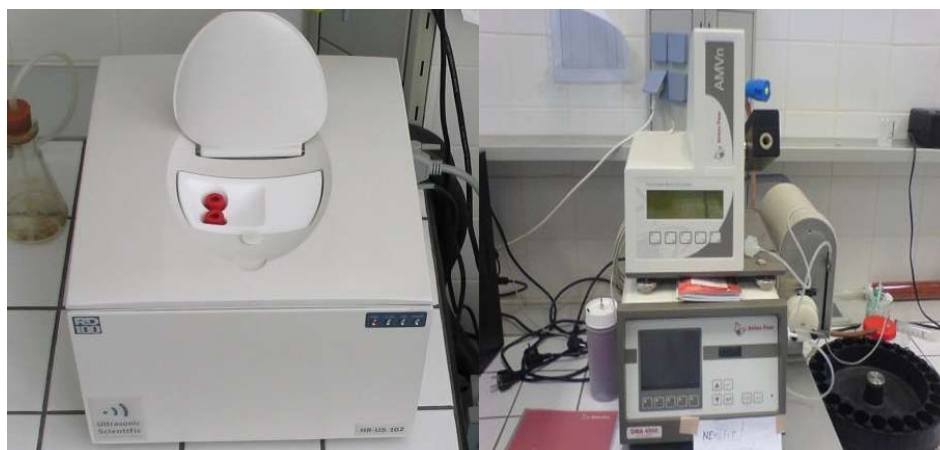
Figure 33: HR-US 102 Ultrasonic spectrometer (left) and Anton Paar DM A 4500 Density meter (right).
