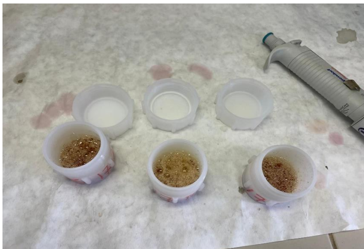
Figure 5: Reaction of the samples after adding Nitric Acid and Hydrogen peroxide
