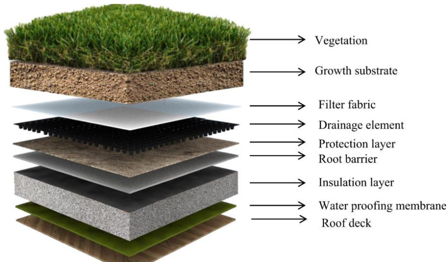
Figure 7. Schematics of different green roof components.
