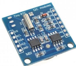
Obr. 5-3 RTC modul DS1307 [36]
