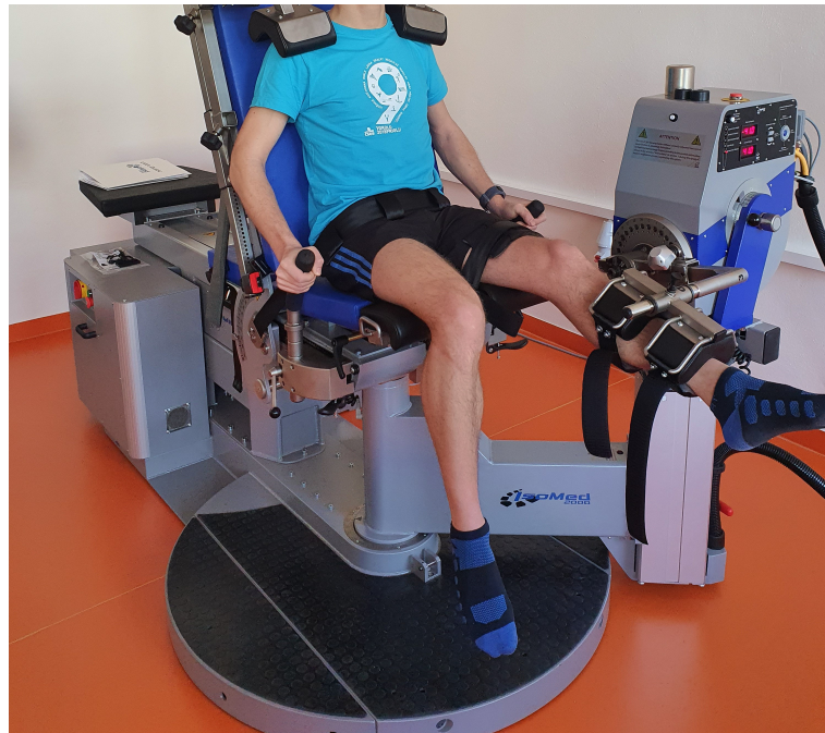
Fig. 2.1: Setting of the dynamometer ISOMED2000. The initial position of the flexion movement.
