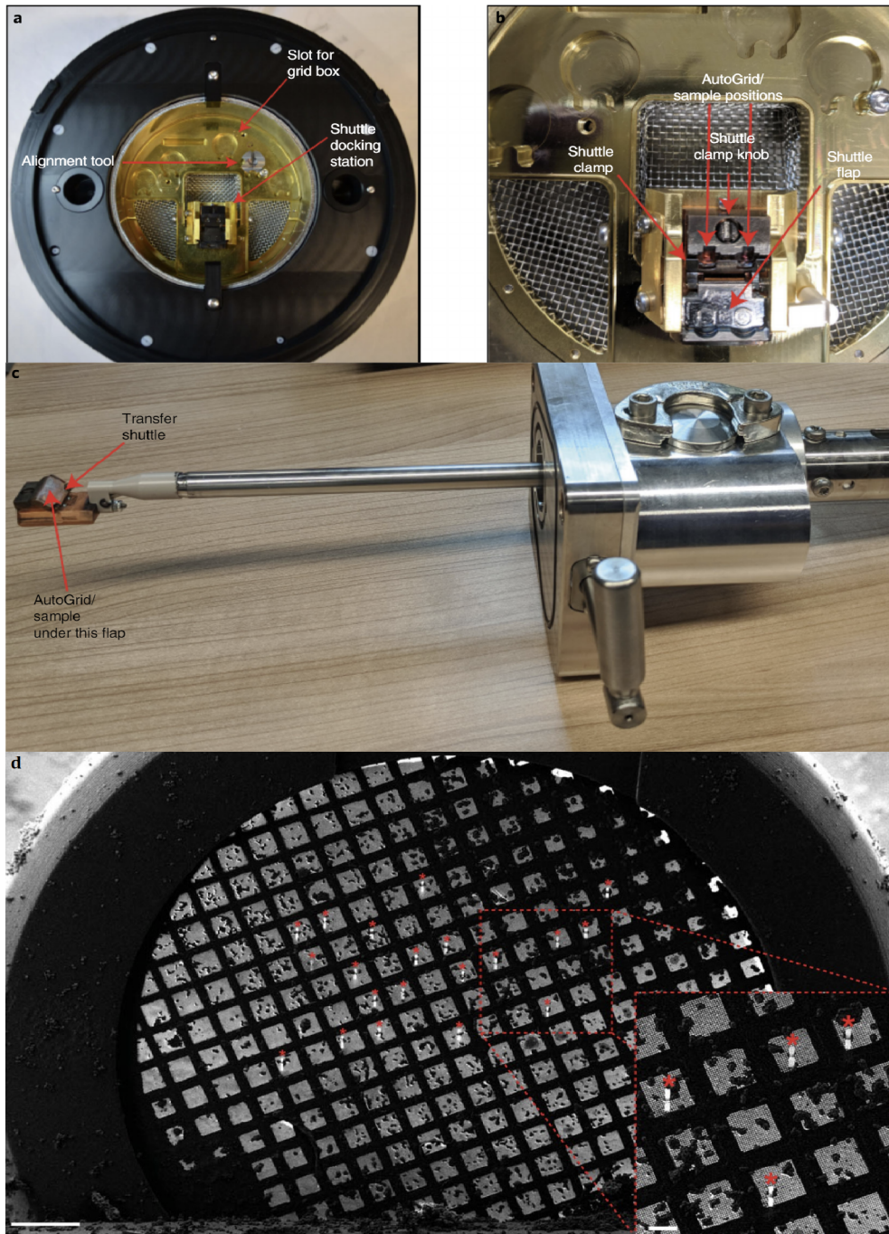
Fig. 1.2: Grid sample preparation. Part (a) depicts the preparation base with cryogen reservoir and sample shuttle. (b) provides closer look to the samples in the preparation base. (c) shows transfer rod to move the sample from preparation base to microscope chamber. (d) depicts the image of the whole grid with the samples. [11]
