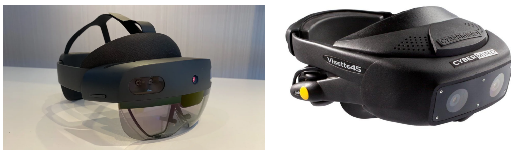
Obr. 2.2: Vľavo: Microsoft HoloLens 2 – optical see-through headset. Vpravo: Visette45SXGA – video see-through headset.
