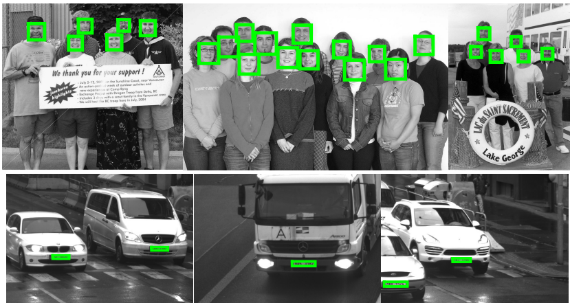
Figure 3.9: Examples of detected objects on selected images from testing datasets for face detection (top) and license plate detection (bottom).
