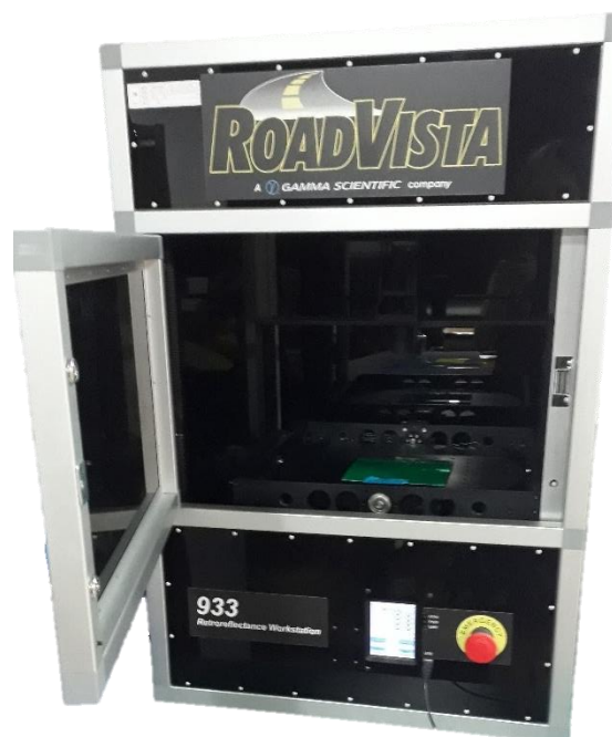
Fig. 38 RoadVista 933 Retroreflective Workstation. Source: Author's foto
