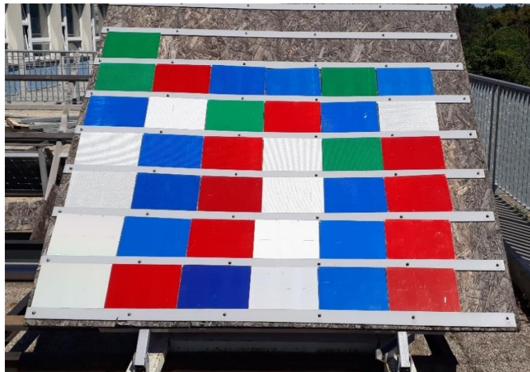
Fig. 36 Test desk with the retroreflective sheeting samples on the roof of the Faculty of Engineering, CULS Prague. Source: Author's photo
