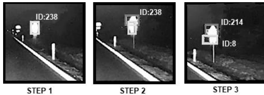
Fig. 67 Demonstration of the issue in recognizing two traffic signs on a single post in three steps. Source: adapted from ADTF development environment, edited by the author
