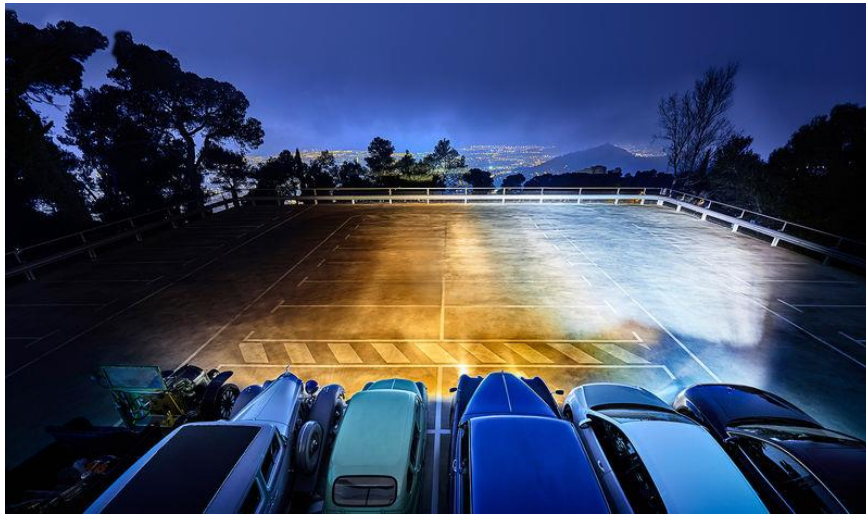
Fig. 21 The evolution of headlights. (From left to right) vehicles by type of optics: carbide (acetylene), simple electric lamps, halogen lamps (two cars in a row), Philips X-tremeVision halogen lamps, and LED matrix headlights. Source: retrieved from “Volvo Car ” (2019)
