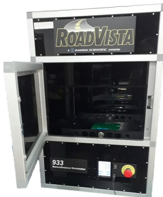
Fig. 38 RoadVista 933 Retroreflective Workstation. Source: Author's foto
