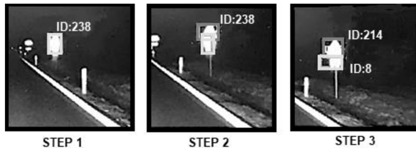
Fig. 67 Demonstration of the issue in recognizing two traffic signs on a single post in three steps. Source: adapted from ADTF development environment, edited by the author
