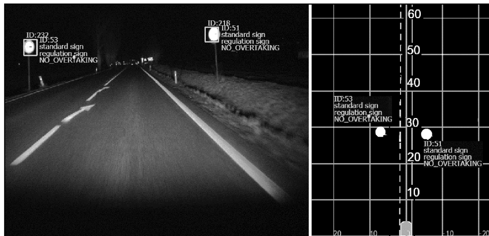
Fig. 40 The screen view of two visualization filters of ADTF. (Left) Video widget with the filter of recognition of traffic signs. (Right) Coordinate graph for determining recognition distance to the signs. Source: ADTF environment
