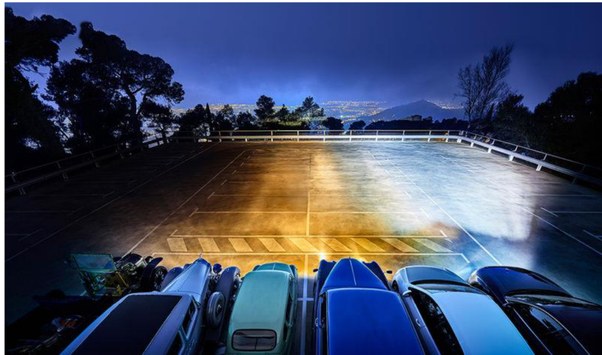
Fig. 21 The evolution of headlights. (From left to right) vehicles by type of optics: carbide (acetylene), simple electric lamps, halogen lamps (two cars in a row), Philips X-tremeVision halogen lamps, and LED matrix headlights. Source: retrieved from “Volvo Car ” (2019)
