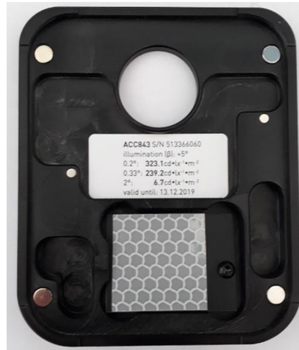
Fig. 37 The front plate of Zehntner ZRS 6060 with the label of the calibration standard (at the top) and calibration standard (at the bottom). Source: Author's foto
