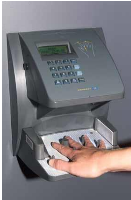
Figure 4 Access control system with a hand geometry reader
