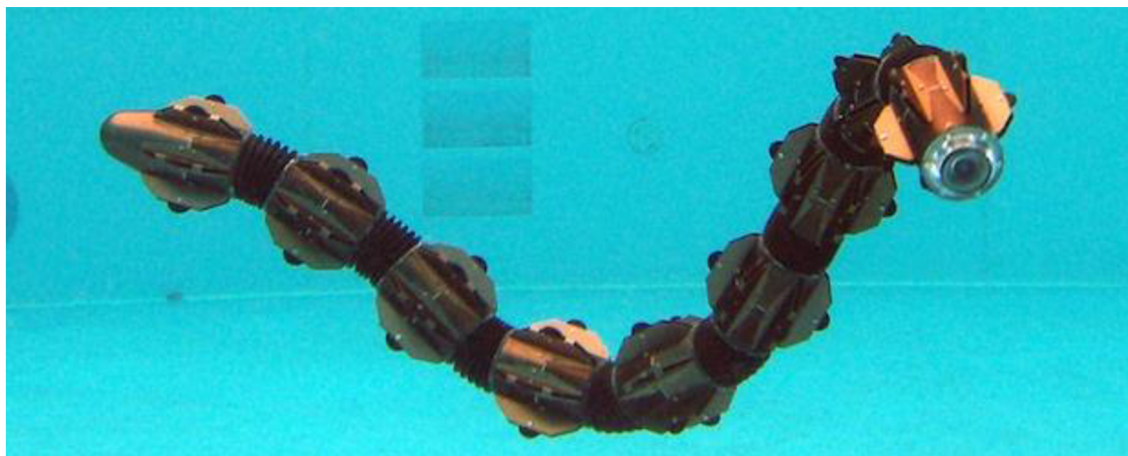
Obr. 21: Vode-odolný robot ACM-R5 [8]
