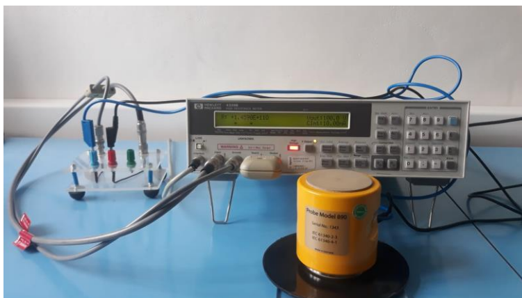
Obr. 7p HP 4339 B High Resistance Meter
