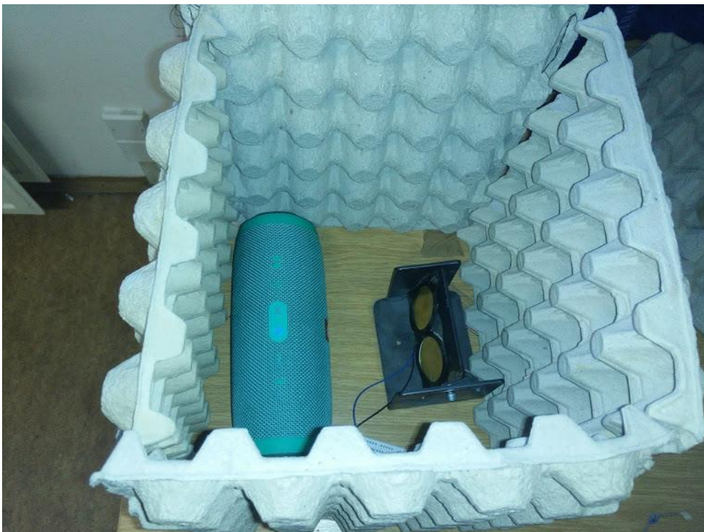
Figure 3-20 : Multiple transducers were placed in en-closer setup.
