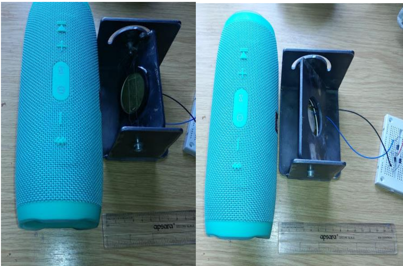
Figure 3-17: Piezoelectric buzzer change in its angle of tilts.
