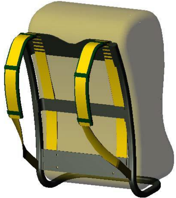
Figure 2-16: schematic of the backpack with piezo-polymer strap
