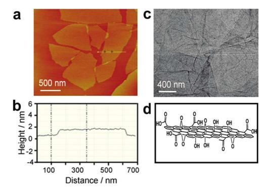
**Figure 6** a) Tapping mode AFM image of oxidized graphene (GO), b) height profile of the AFM image, c) TEM image of the GO, d) schematic model of GO [33]
