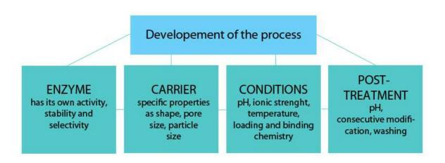
Fig 3 Development of the enzyme immobilization process
