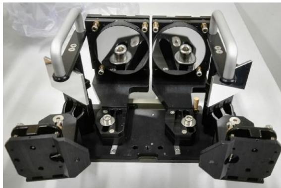
Figure 3.4: The Reflection Unit A515 for External Focus from Bruker which consists of the symmetrical system of mirrors. Half of them is used to focus the beam from the source and then send it focused out through an opening in the spectrometer.
