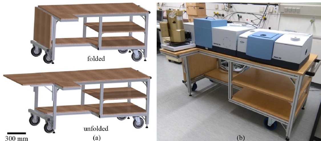
Figure 3.2: (a) 3D model of the folded and unfolded movable table with a scale, (b) final look of the movable table with the spectrometer and its accessories (Infrared Laboratories bolometer).
