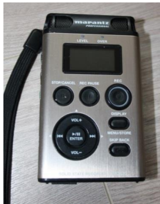
Figure 14: The Marantz Intros PMD620 Portable Media Recorder used in the predator test.
