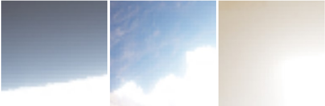
Figure 3.15: Stair-like artifacts in my implementation of the bloom effect. Artifacts become visible around the brightest regions.
