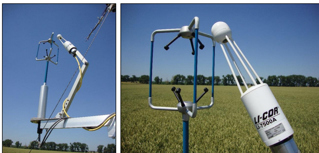
Fig 16 The eddy covariance system an open path CO 2 /H 2 O gas analyser Li7500A (LI-COR Inc., Lincoln, NE, USA) and 3D sonic anemometer WindMaster (Gill, Lymington, UK).
