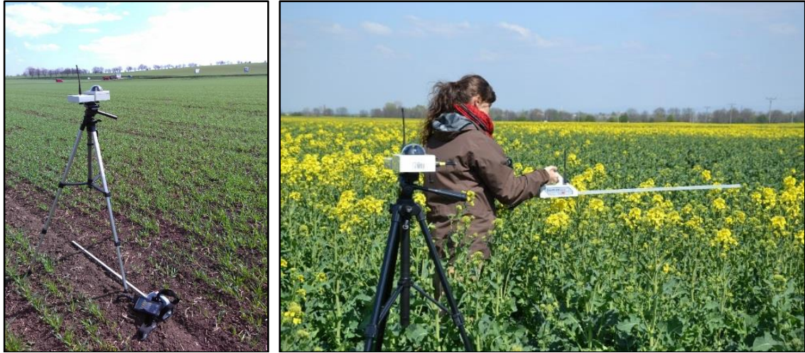
Fig 24 The ceptometer (SunScan by Delta-T Devices, England) (left), field measurement of LAI in oil-seed rape in 2014 in Polkovice (right).
