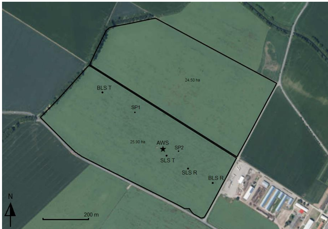
Fig 12 The experimental location and the position of the instrumentation on the field in Polkovice (the Czech Republic) in 2015; star indicates an automatic weather station (AWS), black points indicate scintillometers: boundary layer scintillometer (BLS) and surface layer scintillometer (SLS) letters “T” and “R” stand for transmitter and receiver, respectively. Position of the soil pits (SP1 and SP2). The image was created using https://mendelu.maps.arcgis.com (1. 5. 2016).
