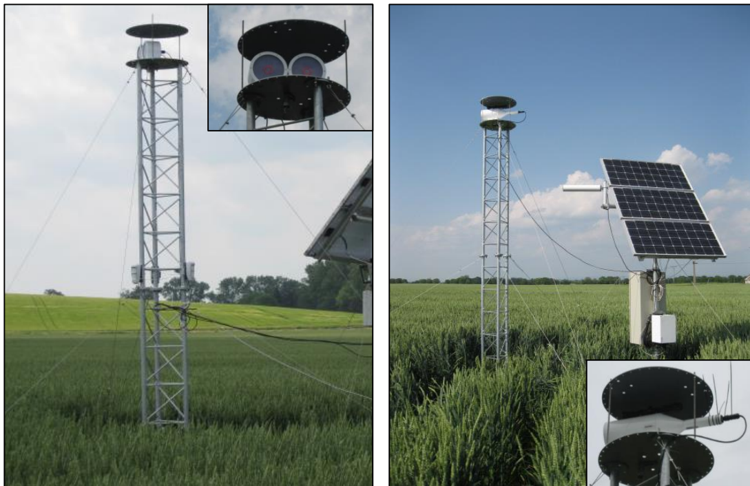
Fig 17 The transmitter (left) and receiver (right) of the boundary layer scintillometer (Scintec, Germany) deployed in winter wheat field in Polkovice 2015.
