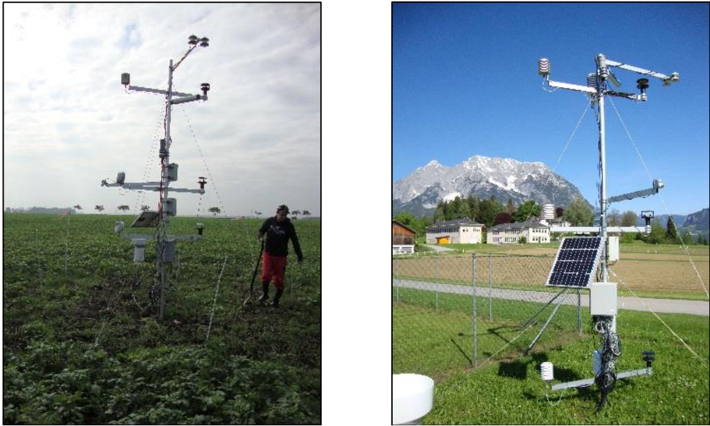
Fig 7 Rutzendorf BLS900 receiver 8.4.2015 (left), BLS900 transmitter 13.11.2014 (right).
