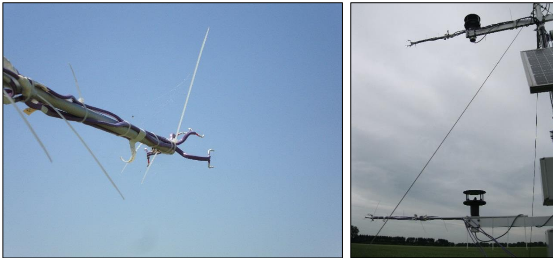
Fig 21 Thermocouples for the surface renewal method (left), position on the arms of AWS (right).
