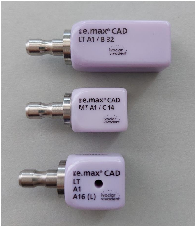
Figure 22: Photo of IPS e.max CAD. Different sizes, translucencies and types of blocks.
