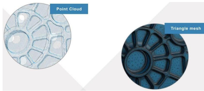
Figure 4 Cloud points and polygonal mesh triangles [3]
