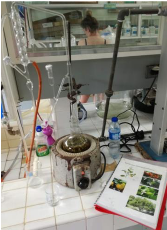
Hydrodistillation of C. microcarpa , Baybay, Philippines (Fiserova, 2018) from @lee_lab_prague
