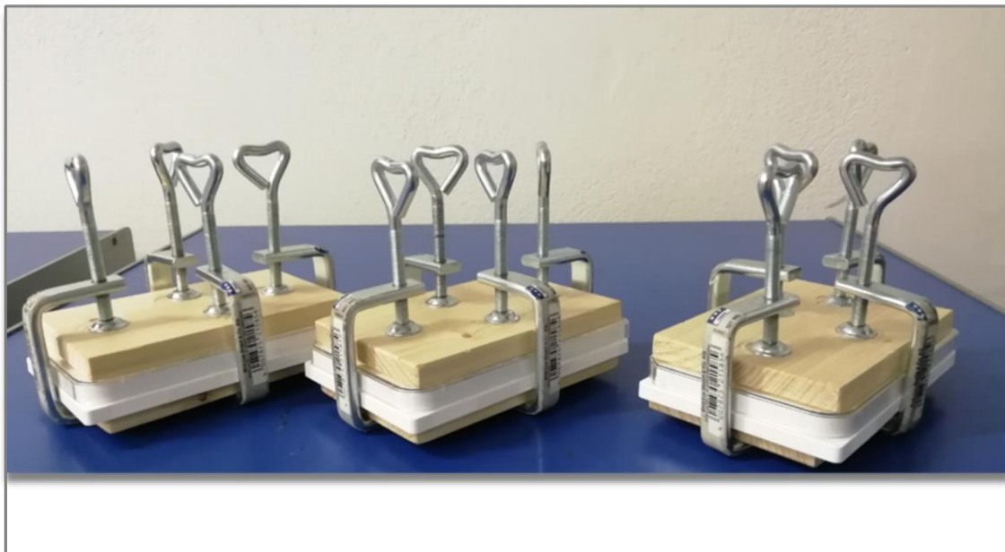
Figure 2: Clamps and wooden pads for fastening lids and plates together prior to incubation
