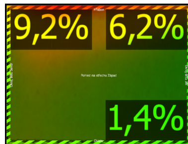
Fig. 6.3: Simulated shading on roof section 4
