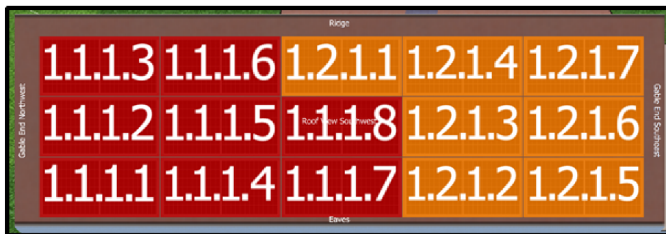
Fig. 10.6: Module placement of the balanced variant
