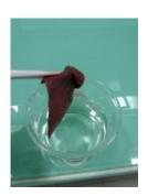
(b). Photographs of chloroform removal from underwater surface
