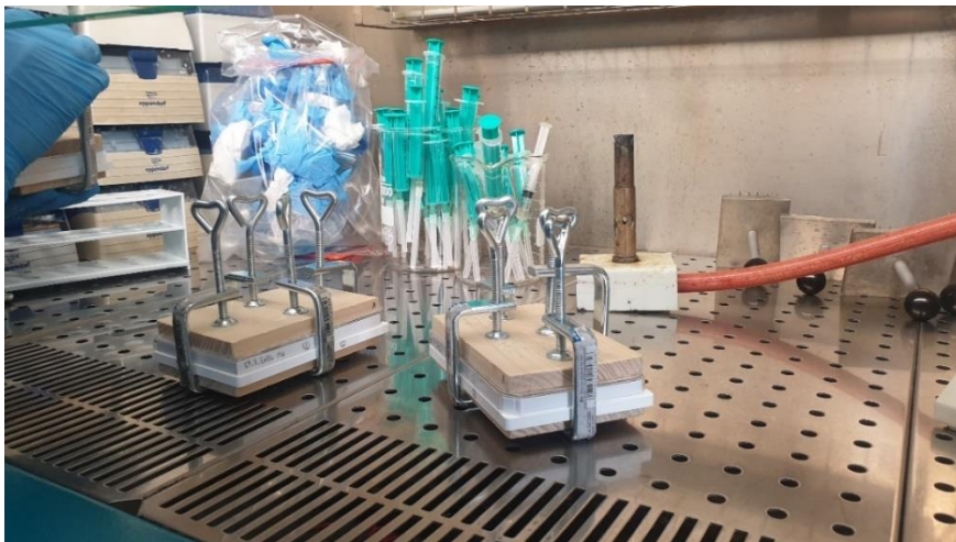
Figure 15. The clamps (Prague, Lux Tool, CZ) were utilized for fastening lid and plate together.
