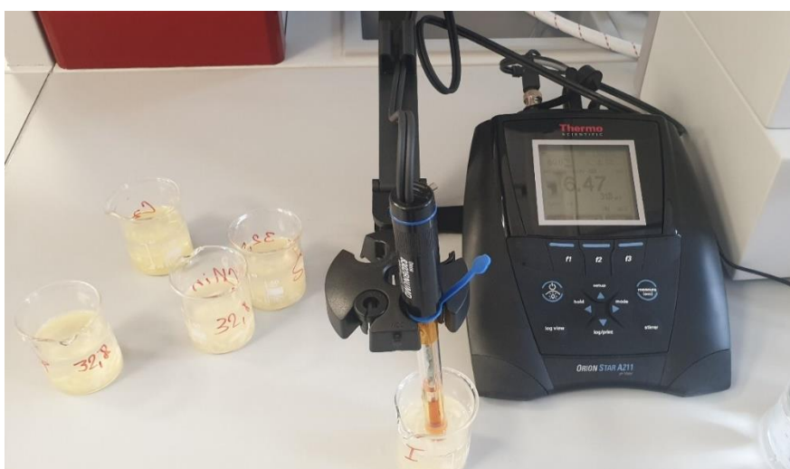
Figure 19. A schematic diagram showing pH measurement of a garlic sample in CZU-FTA lab.
