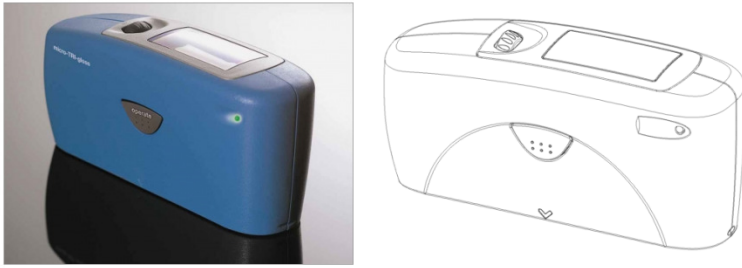
Figure 38 Micro-TRI-gloss \mu - BYK Gardner. Right – scheme of device. Small arrow points out mark for measure aperture. 118
