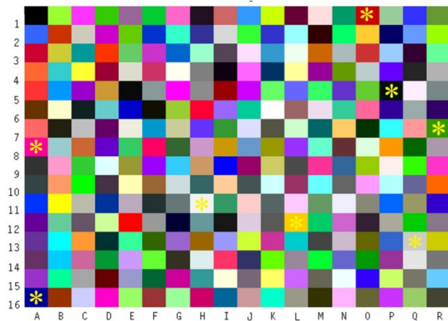
Figure 49 Measured patches for colour change on I11.5 test target after varnish application are marked with yellow star.
