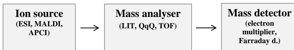
Figure 18: Mass spectrometry scheme (Ekman *et al.*, 2009)
