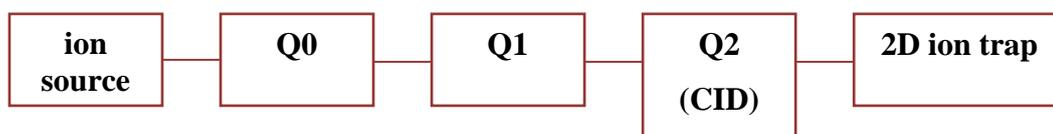
Figure 21: Simplified scheme of Q-Trap (created by <http://msr.dom.wustl.edu/>, 2015)
