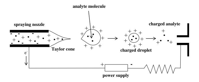
Figure 19: Electrospray ionization scheme (created by http://www.hindawi.com, 2015)
