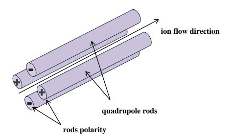
Figure 20: Quadrupole scheme (created by Gross, 2004)
