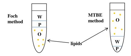
Figure 16: Phase and lipid distribution in Folch and MTBE extraction methods, where O = organic phase, W = water phase, P = precipitant (Matyash *et al.*, 2008)
