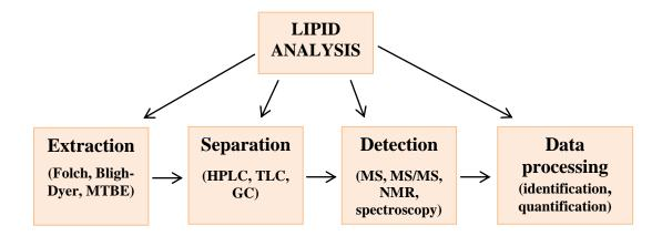
Figure 15: Lipid analysis scheme (Cajka et Fiehn, 2014; Carrasco-Pancorbo et al., 2009)
