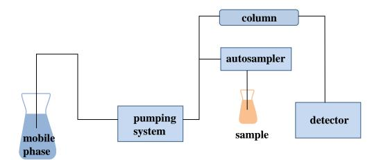
Figure 17: HPLC scheme (created by <u>http://www.waters.com</u>, 2015)
