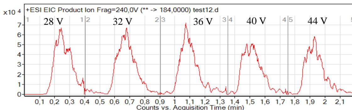
Figure 27: Collision energy test for PC (16:0/16:0) in ESI-
