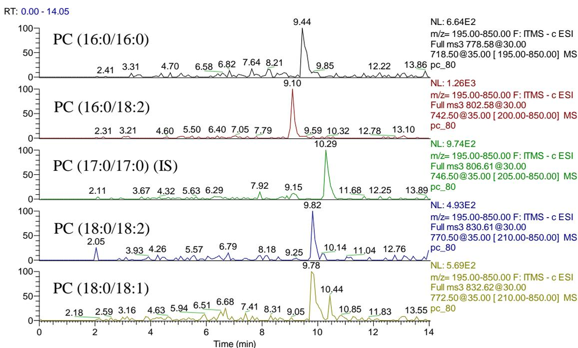
Figure 33: ESI- MS<sup>3</sup> chromatograms of the four 500 nM PC standards + 1µM IS in MeOH
