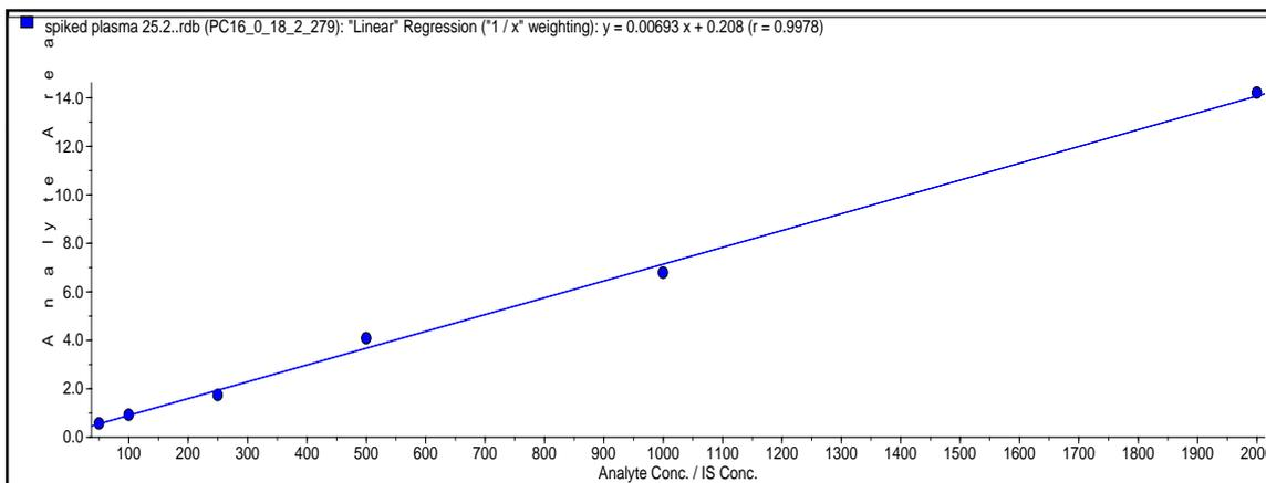
Figure 36: Calibration curve of PC (16:0/18:2) in spiked plasma
