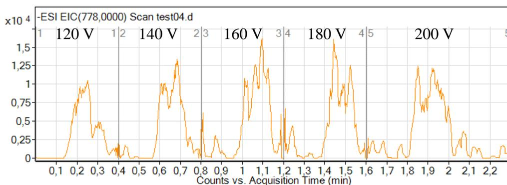
Figure 26: Fragmentor voltage test for PC (16:0/16:0) in ESI-
