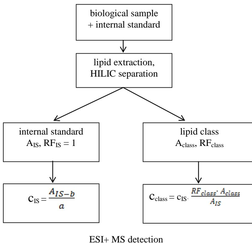
Figure 24: Scheme of lipid class quantification by Cifkova *et al.* (2012), where RF = response factor, IS = internal standard, A = peak area c = concentration, a = slope, b = intercept
