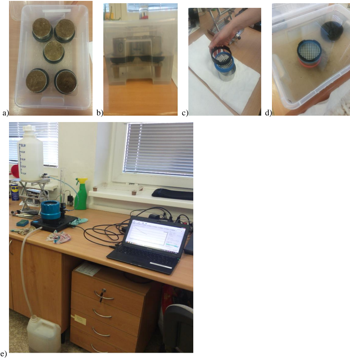
Figure 9. Photo-documentation of the KSAT measurement a) Samples before saturation b) Samples during saturation c) Fittings before measurement d) After fittings and before transferring to the measuring dome e) Complete set-up during measurement.
